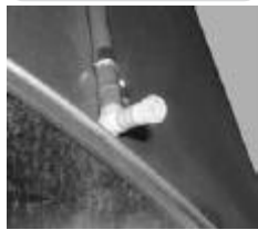
Measuring connector in inlet cone Hose pipe to connecting piece in the side wall Connecting piece (external diameter of 6mm) for the pressure measurement
