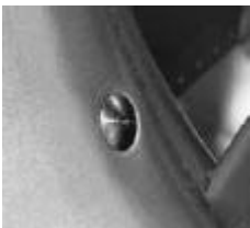
Measuring connector in inlet cone Hose pipe to connecting piece in the side wall Connecting piece (external diameter of 6mm) for the pressure measurement
